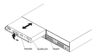
Figure 49. Removing and replacing a controller
